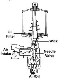
Lighter duty pumps use wicks to regulate oil flow, while heavy-duty oilers are available for those applications where large units are operating continuously under harsh conditions.
