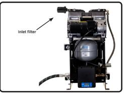
6 If using, attach the supplied connecting hose to the 3/8" threaded outlet. Secure flange nut on hose using adjustable wrench. Remove the plastic plug from the compressor head port, install the provided inlet filter in the same port. hand tightening.
