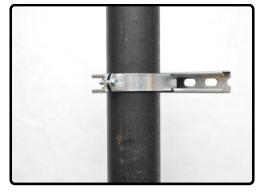
Use the included (shipped loose) top channel strut, install using the proper sized clamps for the riser pipe diameter. A kit of clamps is included with every unit. Make sure the strut channel is level and secure clamp bolt & nut.
