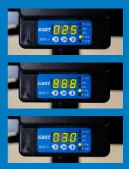
To adjust the cut-out pressure, press the UP arrow once. The P OFF light will flash.
