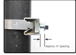
Ensure there is enough space between the bolt head and channel strut to allow the system frame to mount in between.
