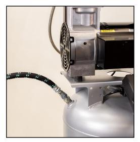
If using, attach the supplied connecting hose to the 3/8" threaded outlet. Secure flange nut on hose using adjustable wrench. Remove the plastic plug from the compressor head port, install the provided inlet filter in the same port, hand tightening.
